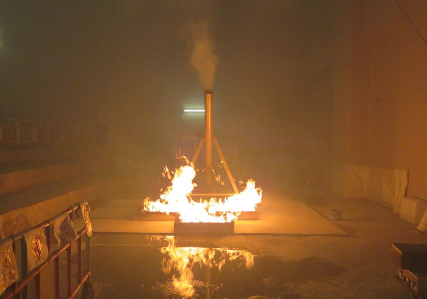
Motorized Fire & Smoke Damper failed to operate effectively during the test
